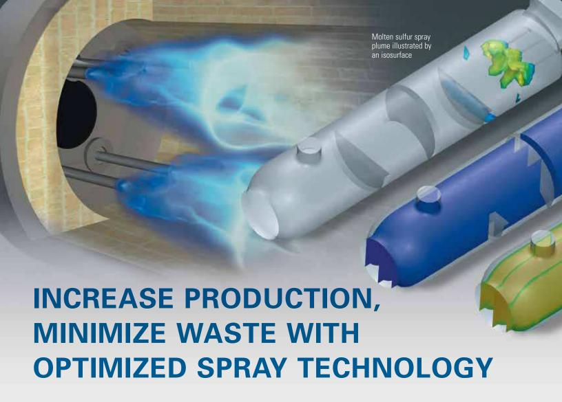
Achieving the proper sulfur droplet size and maintaining the proper temperature are the keys to maximizing production and furnace efficiency.
