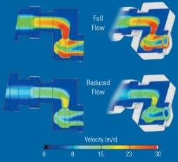
At the reduced flow conditions, the sulfur polymerizes inside the BA WhirlJet gun as the temperature rises above 305.6°F (152°C). A skin forms and grows thicker over time eventually plugging the gun.
