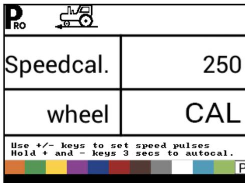
NOTE: When the Automatic Calibration Mode is activated, no other functions are possible until the console receives Pulses for calibration. To deactivate the Automatic Calibration Mode, press the PLUS **+** button until a number is displayed.
