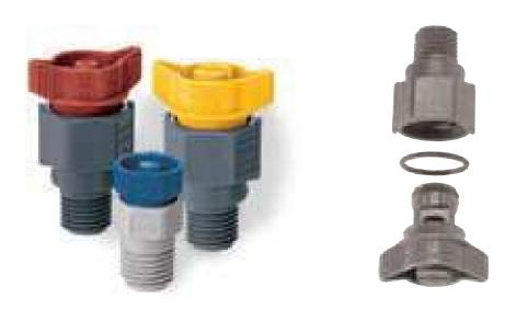
**ProMax® QuickJet® nozzles** feature a quick-connect design that decreases maintenance time and reduces costs. The nozzle body stays on the header and only the spray tips are replaced. Spray tips are removed and installed by hand and spray patterns are automatically aligned.
