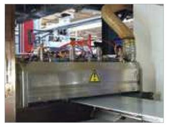
All nozzles are contained in the coil lubricator unit. An oil mist extractor is used in the coil lubricator to prevent misting and worker inhalation problems. The system also features oil recirculation to minimize overall lubricant usage. Automatic solenoid valves ensure excess oil is returned from the coil lubricator back to the correct supply tank. The oil is filtered on the suction lines to ensure no contaminants enter the system.
