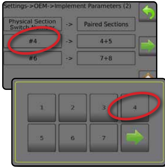
Figure 3-43: Physical section switch number
