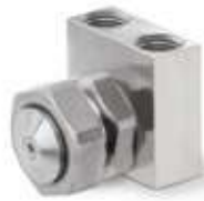
6552-1/8JAC – Miniature design is only 1/2" thick with a 1-5/32" by 1-1/4" rectangular face. The air and liquid inlets on the same side of the nozzle body – 90° to the spray direction
