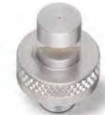
QSTK Spray Tip Miniature version Flow rates below 1 gpm at 40 psi (3.9 lpm at 2.8 bar) Use with seal and QJJS body
