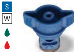
QPHA Spray Tip – Blue QPHA-10 1.0 gpm (3.8 lpm) QPHA-12W 1.2 gpm (4.6 lpm) Use with QPPA body
