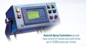
**Precision Spray Control (PSC)** involves switching spray nozzles on and off very quickly in order to control the flow rate. This cycling takes place so quickly that the flow often appears to be constant. PSC requires the use of electrically-actuated nozzles and an AutoJet spray controller.
