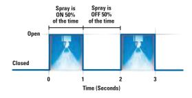
**Precision Spray Control (PSC)** turns nozzles on and off quickly to control flow rate. This cycling is so fast that the flow often appears to be constant. Unlike traditional nozzles, which require a change in liquid pressure, PSC allows the pressure to remain constant and enables flow rate changes without changing the spray angle or drop size.
