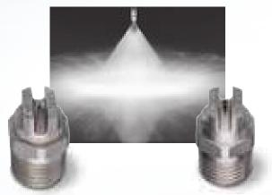
WashJet® spray nozzles (left) provide powerful cleaning performance. These nozzles produce a high impact spray and feature a maximum operating pressure of 3000 psi (207 bar). VeeJet® nozzles (right) with tapered-edge flat spray patterns are typically installed on a spray header. Overlapping spray distribution ensures uniform coverage. In this application, the entire steel plate is thoroughly rinsed as it passes under the header.
