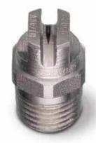
**VeeJet® nozzles** produce a thin, tapered-edge, rectangular spray pattern with medium sized drops and higher impact. Positioned to the side of the rail cars, the higher impact spray penetrates the falling iron ore and provides effective dust control.
