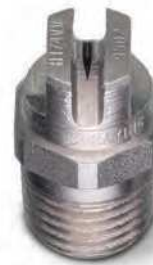
H-VV and H-VVL 1/8" to 1/4" male conn. Flow rates below 1 gpm at 40 psi (3.8 lpm at 2.8 bar) H-VVL includes integral strainer
