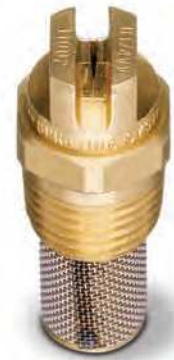
H-VV and H-VVL 1/8" to 1/4" male conn. Flow rates below 1 gpm at 40 psi (3.8 lpm at 2.8 bar) H-VVL includes integral strainer
