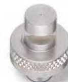
QSTK Spray Tip Miniature version Flow rates below 1 gpm at 40 psi (3.9 lpm at 2.8 bar) Use with seal and QJJS body
