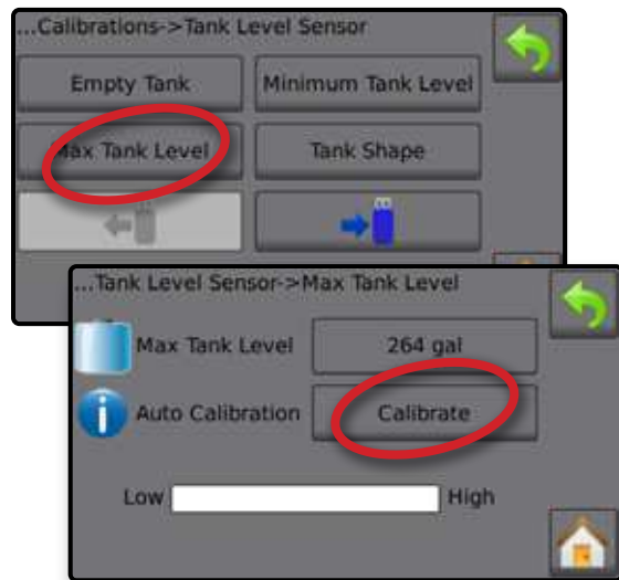
Figure 3-32: Tank Level Sensor – Maximum Tank Level
