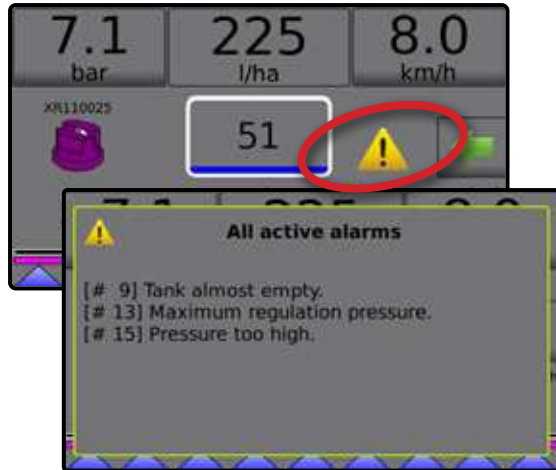
Figure 2-20: Active Alarm Warning List
