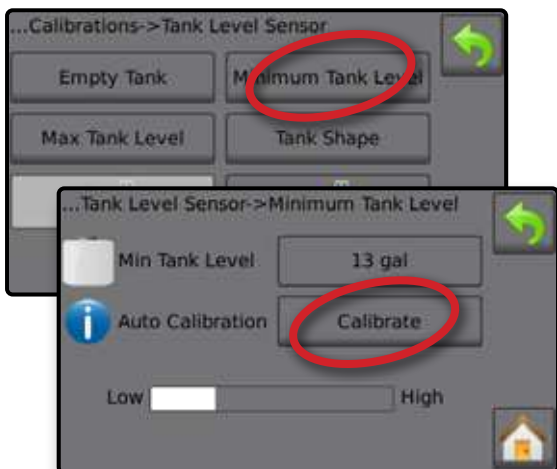
Figure 3-30: Tank Level Sensor – Minimum Tank Level
