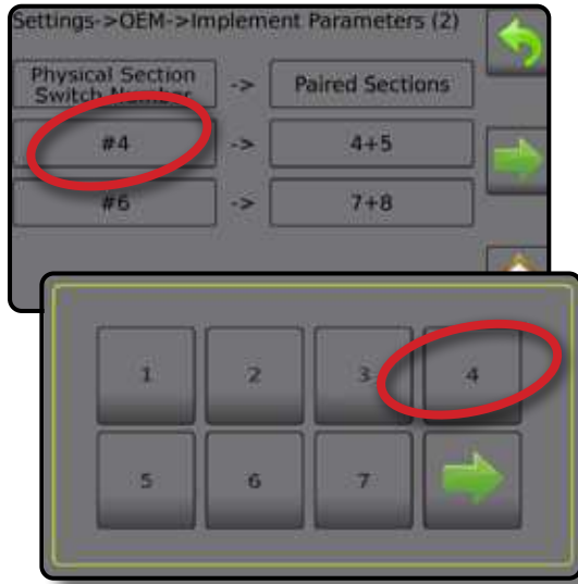
Figure 3-43: Physical Section Switch Number
