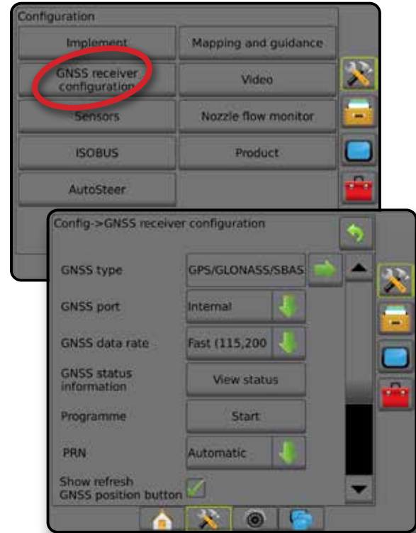
Figure 4-16: GNSS receiver configuration options
