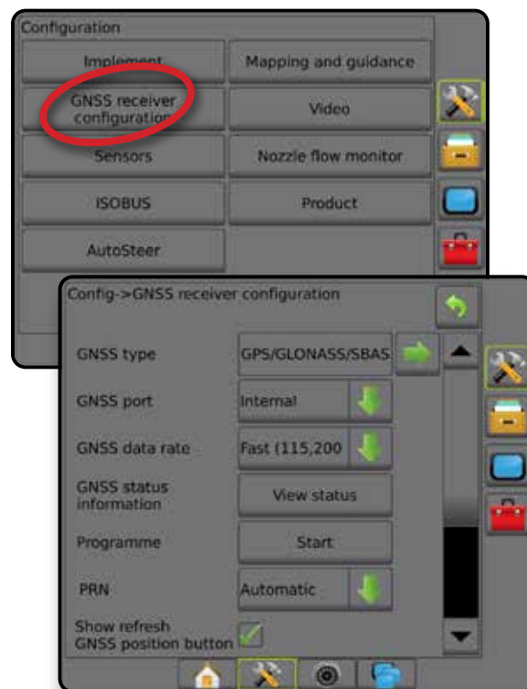
Figure 5-1: GNSS receiver configuration options
