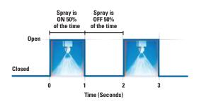
Precision Spray Control (PSC) turns electrically actuated PulsaJet nozzles on and off guickly to control flow rate. With traditional nozzles, flow rate adjustments require a change in liquid pressure, which also changes the nozzle's spray angle/coverage and droplet size. With PSC, pressure remains constant, enabling flow rate changes without affecting spray performance. This reduces the use of costly coatings by applying the proper volume directly on the cables.
